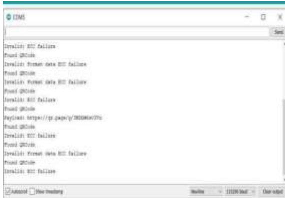
Fig 4.7. Output of the scanner unit in IDE
