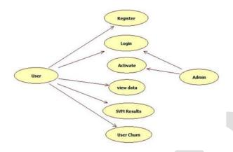
A use case diagram in the Unified Modelling Language (UML) is a type of behavioural diagram defined by and created from a Use-case analysis. Its purpose is to present a graphical overview of the functionality provided by a system in terms of actors, their goals (represented as use cases), and any dependencies between those use cases. The main purpose of a use case diagram is to show what system functions are performed for which actor. Roles of the actors in the system can be depicted. [14]
