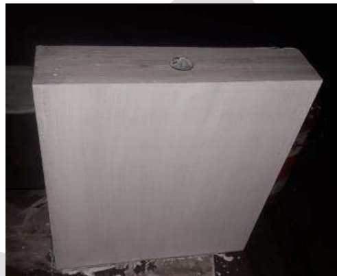
Fig. 6: Specimen 290x290x70 coated with delta glaze coating
