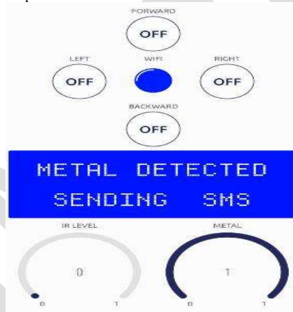
Fig 6:Robot Detecting metal shown in Blynk app
