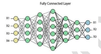
In the above diagram, the feature map matrix will be converted into the vector such as **x1**, **x2**, **x3**... **xn** with the help of fully connected layers. We will combine features to create a model and apply the activation function such as **softmax** or **sigmoid** to classify the outputs as a car, dog, truck, etc.
