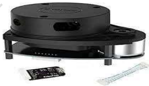
Fig. 4. LiDAR sensor used for mapping and obstacle detection.
