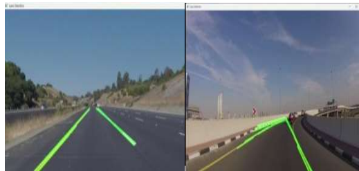
Fig. 3. Detection output for a solid yellow left lane and for a road car view.
